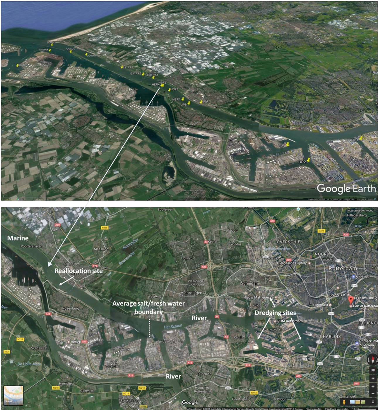
Figure 1 Port area for sediment reallocation (top) versus the larger port area upstream of the reallocation site (bottom)
