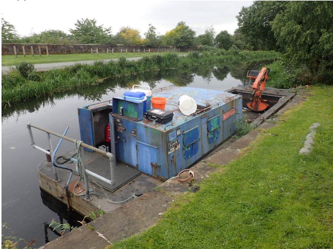
(b) Hydraulic clam-shell used for sampling sediment (as semi-solid sludge).
