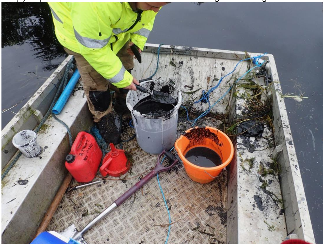
(c) Liquid sediment recovered and weed issues using Van Veen grab.
