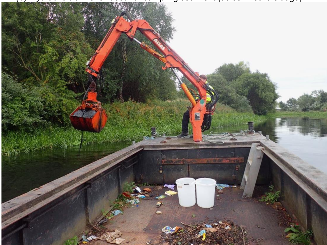
(b) Hydraulic clam-shell used for sampling sediment (as semi-solid sludge).
