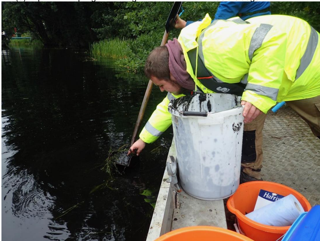
(d) "Spoon" sampling illustrating recovered sediment as a sludge.
