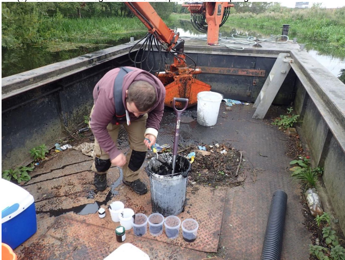
(c) Sediment homogenisation and replicate subsampling.
