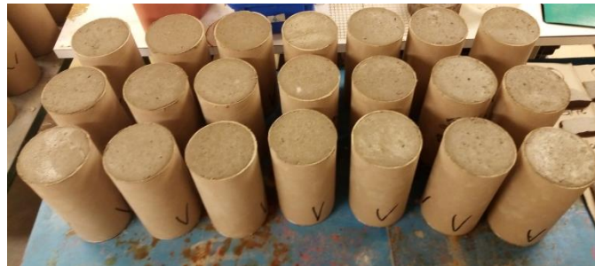
Figure 2. Cylindrical concrete specimens 11 cm × 16 cm.
