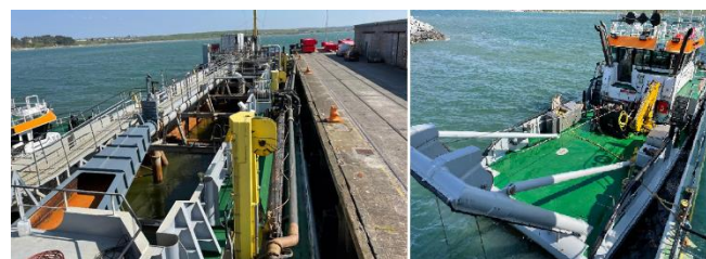
Figure 8. Hydraulic Dredger Marbury (left) and Plough Dredger (right) used at the Port of Fenit
