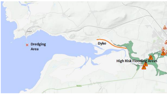
Figure 9. Proposed Dyke Location and Areas of High Flood Risk in Tralee Bay
