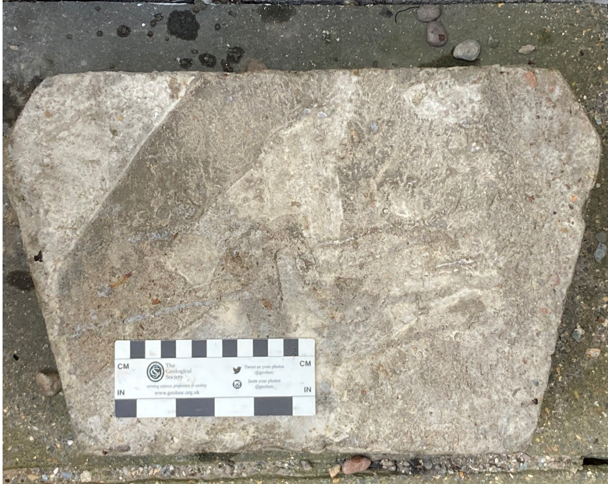
30kg concrete block for retaining wall – flood control
