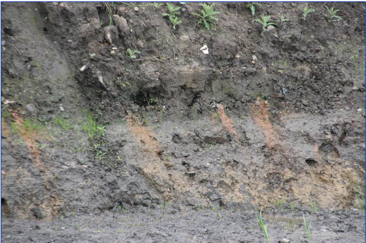
Figure 42. Evidence for the ingress of soil water from the up gradient part of the site.
