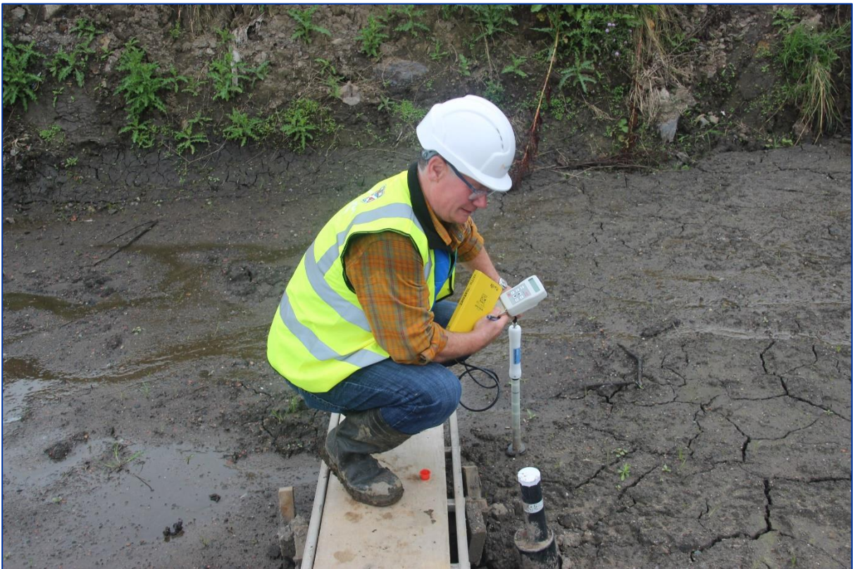
Figure 40. In-situ measurement of soil moisture at six horizons using soil moisture probe and moisture meter.
