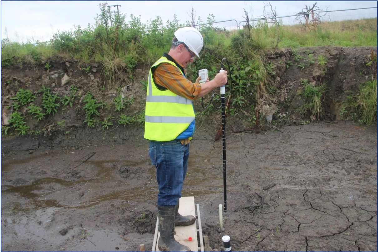
Figure 39. Moisture probe (PR2/6) prior to insertion into pre-installed fiberglass sleeve.
